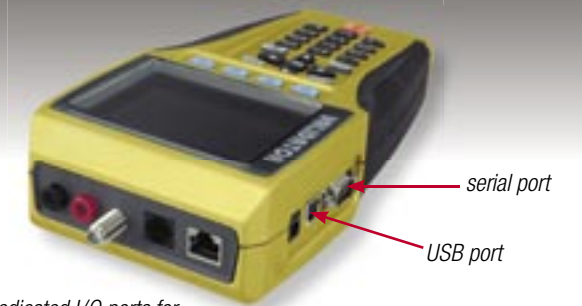
dedicated I/O ports for network, telephone, coax and paired cables
