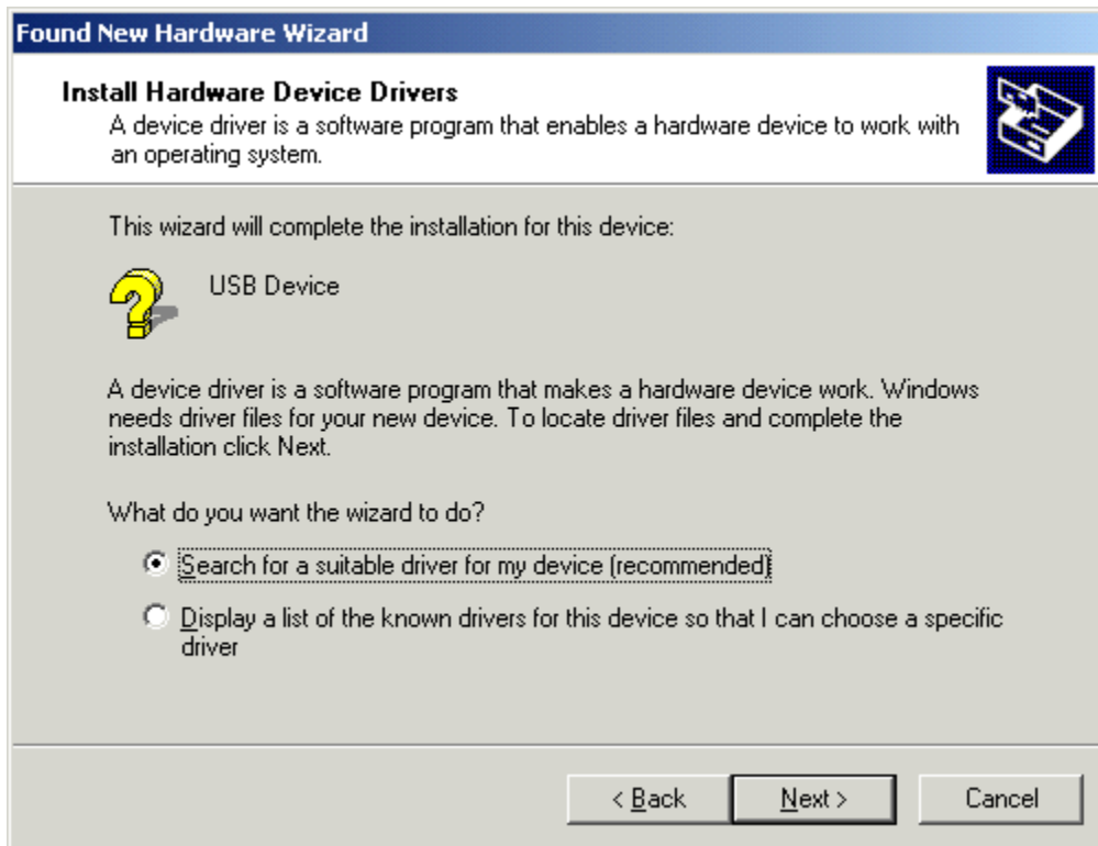
Figure 38. When asked What do you want the wizard to do? , select "Search for a suitable driver for my device" and click "Next" .
