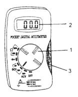
Rotary Switch : Switch for selecting measurement functions & ranges as well as the
