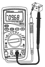
" \( \Delta \)" means the maximum current of mA socket is 400mA, the maximum current of 10A socket is 10A, over-current will destroy the fuse (10A range unfused).
