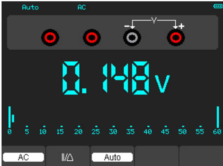
Figure 4-6: AC voltage Measurement
