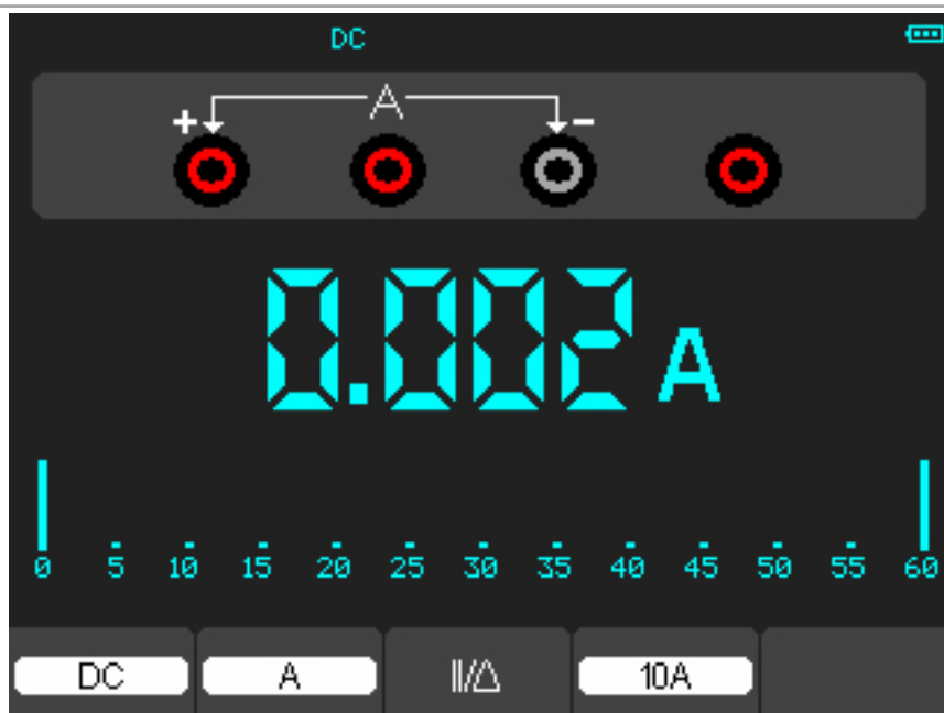
Figure 4-8 DC Current Measurement for 10A
