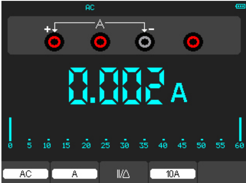
Figure 4-10 AC Current Measurement for 10A
