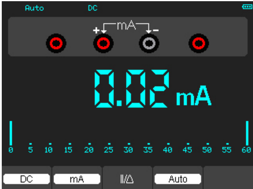
Figure 4-7 DC current Measurement for 600 mA
