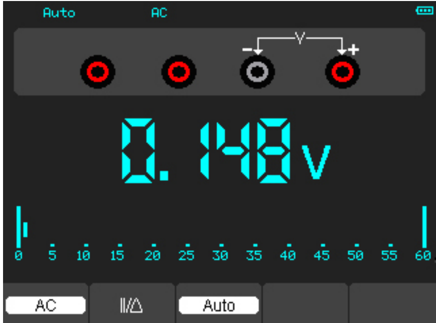
Figure 4-7 AC voltage Measurement
