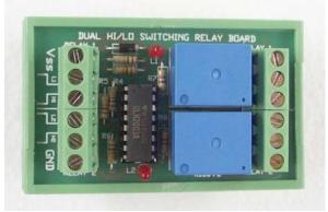
In this Version 2 PCB we have increased the board size to fit in a PCB carrier as shown in the photo. This DIN rail carrier is not supplied. It is just to show you. We have also added an LED across each relay to show when it is activated.
