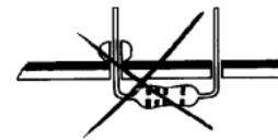
3- Trim excess leads as close as possible to the solder joint
