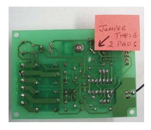
Connect the other side of the tact switch to ground as shown. Use an offcut fron resistor leg. See it at
